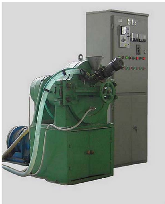
Figure 1. Digital camera picture of pan-mill type reactor. [Color figure can be viewed in the online issue, which is available at wileyonlinelibrary.com.]
